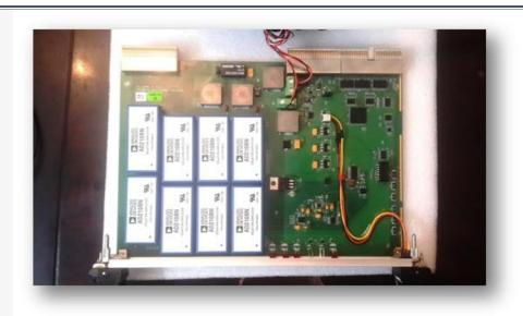
SPARTAN 6 FPGA based cPCI Interface based Industrial grade 6U, 4HP, 66MHz, 8 Channel K type Thermocouple Card.
